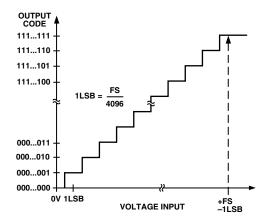
Figure 5. ADC Transfer Function
